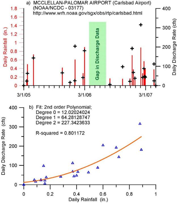
**Figure 3.** Relation between rainfall and discharge rate of Agua Hedionda Creek: a) Rainfall (red bars) & daily discharge Agua Hedionda Cr. (black crosses from Tetra Tech, 2007). b) Hydrographic rating curve (red) from 2nd order polynomial fit to flow rate vs rainfall data (blue diamonds).
